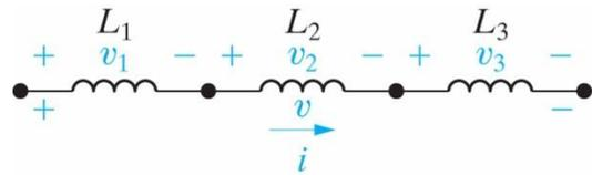
$$v = v_1 + v_2 + v_3 = (L_1 + L_2 + L_3) \frac{di}{dt}$$
