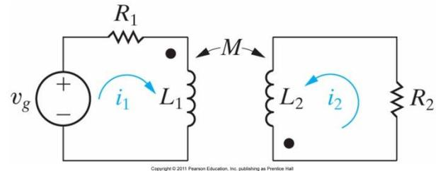
**Rule**: When the reference direction of the **current enters** the dotted terminal of a coil, the reference polarity of the voltage induced in the other coil is **positive** at its dotted terminal
