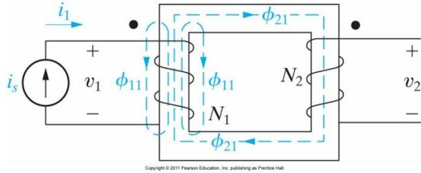
The total flux linking in coil 1
