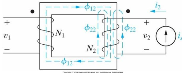
The total flux linking in coil 2
